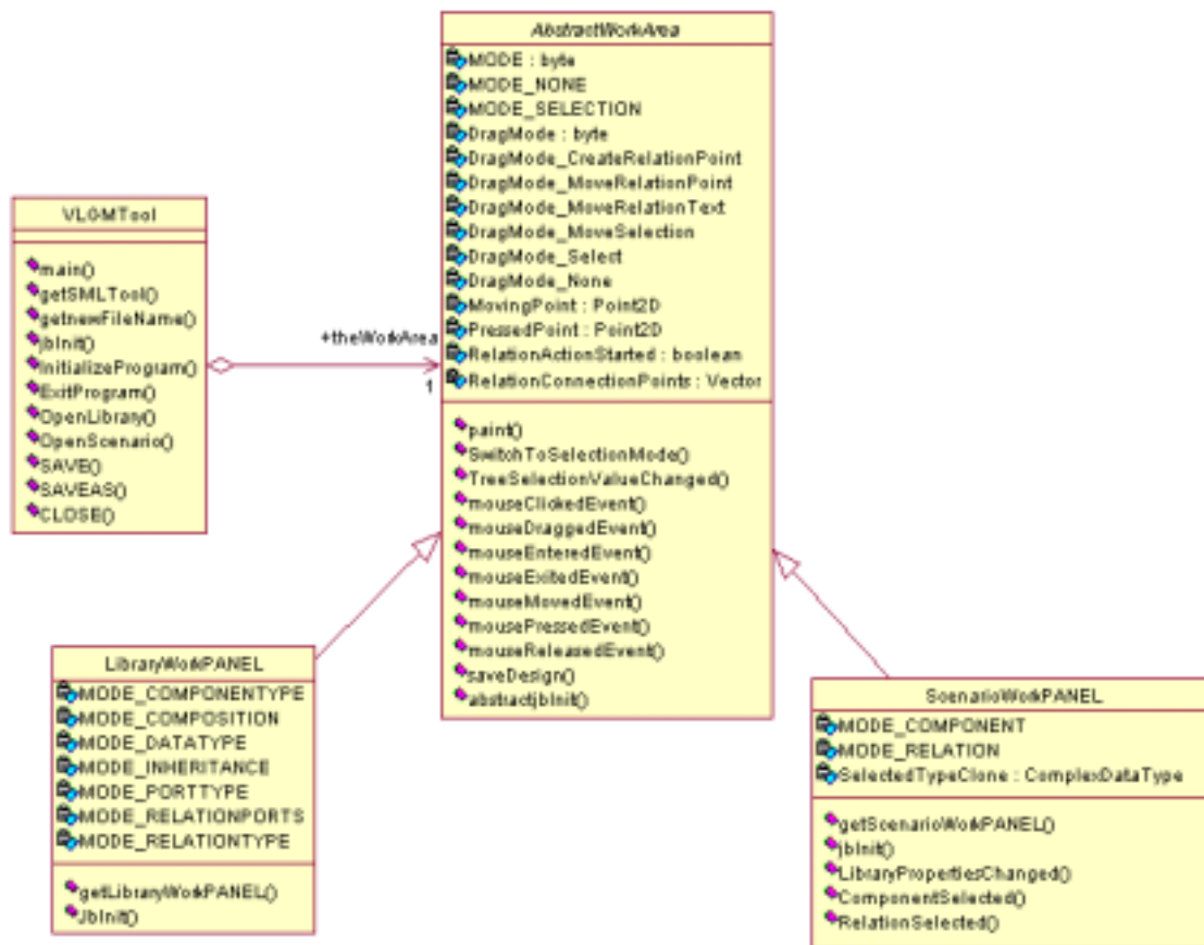
Figure 49. Class Diagram of Main Design Area
